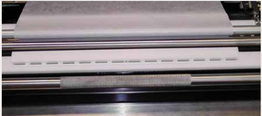
RapidClean is a high-speed under-stencil cleaning system offered on MPM Momentum series printers. RapidClean is the fastest stencil cleaning solution available.
